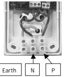
Attach the phase (brown), neutral (blue) and earth (yellow/green) wires on the IntelliSwitch socket to the house supply phase (red), neutral (black) and earth (green) with connector block (supplied).
