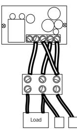
Attach the supplied 3-way connector block to the IntelliSwitch<sup>™</sup> as shown.
