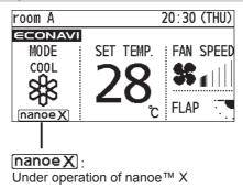
nanoe™ X For a freshness and cleaner environment nanoe™ X generates negative ions using the air in the room to give a healthy air. It also reduces the smell in the room, and constrains propagations of mold and bacteria.
