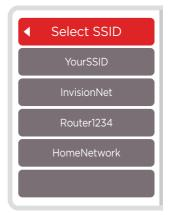
The routers in the list will be different to the ones displayed above as they are the 5 strongest Wi-Fi signals found near to the touchscreen display. This screen will refresh every 10 seconds, so if the router you are looking for does not appear, wait for the next scan. Select the one you
