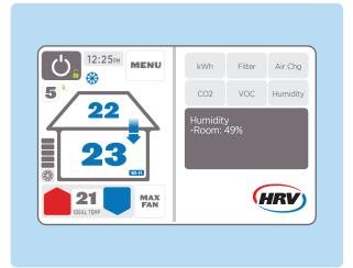
Once no smoke is detected, the HRV system will automatically stop the alarm and return the HRV system to the main screen and normal fan operation (shown here on left).
