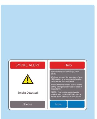
'SMOKE ALERT' is displayed with a 'beeping' sound, within 10 seconds of the smoke alarm being activated (shown here on left).
